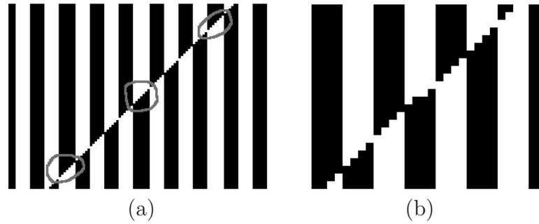
Figure 7.3: Typical errors in binary computer-generated holograms. (a) An example of a holographic pattern with varying fringe spacing. Most of the fringes are six pixels wide, whereas the three circled fringes are seven pixels wide. (b) An example of a holographic pattern with a single-pixel displacement error in the phase discontinuity line resulting from a poorly chosen offset for the  $x$ - $y$  grid alignment.
