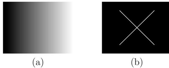
Figure 7.4: Two test images for characterising the slide film and the Polaroid slide writer: (a) a smoothly varying grey scaling—to check the response of the film and the exposure levels required; (b) image of a square cross ( $2048 \times 2048$  pixels)—allows accurate measurement of pixel size and astigmatism.
