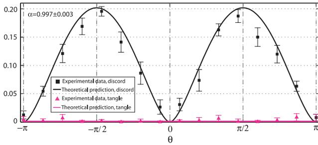
FIG. 4 (color online). Nonclassical correlations generated by our DQC1 algorithm. Discord and tangle are derived from the reconstructed density matrices measured at the algorithm output for  $\alpha = 0.997 \pm 0.003$  [Fig. 3(a)]. Discord is calculated by optimizing over all 1-qubit projective measurements on qubit  $c$ , Fig. 1 [26]. Theoretical predictions are calculated using measured input states and assuming perfect circuit operation.
