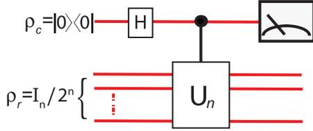
FIG. 1 (color online). Algorithm for estimating the normalized trace of the unitary operator  $U_n$ , using deterministic quantum computing with 1-qubit (DQC1).  $I_n$  is the  $n$ -qubit identity. Repeated running of the circuit and measurement of qubit  $c$  in the Pauli  $X$  ( $Y$ ) basis yields an estimate of the corresponding expectation value, from which one can derive the real (imaginary) part of the normalized trace ( $\text{Tr}[U_n]/2^n$ ).
