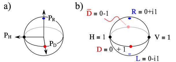
FIG. 6: Poincaré sphere. a) a set of measurement axes that define the sphere. b) positions of a range of polarisation (log-ical) states on the sphere.
