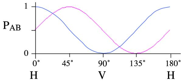
FIG. 5: Coincidence probability vs Bob's analyser setting. Alice is analysing in the D/D̄ (45°/135°) basis.
