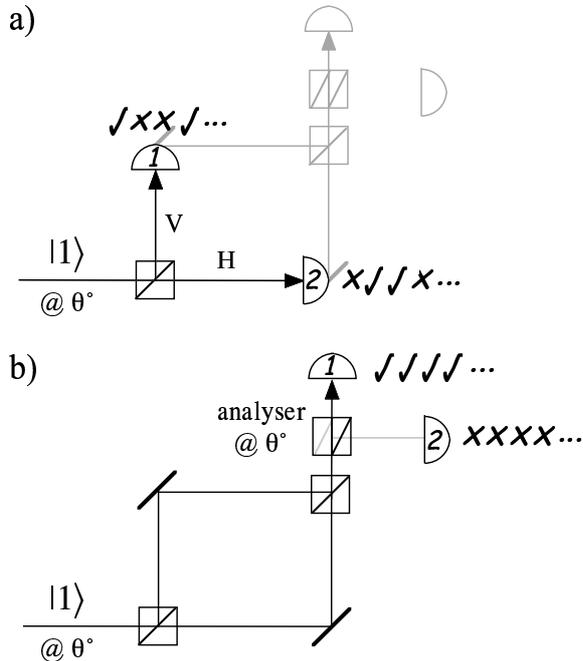
FIG. 2: Qubits carry phase information. a) a polarisation qubit,  $\theta^\circ$ , incident on a polarising beamsplitter. b) a polarisation qubit incident on a polarising interferometer. The qubit is passed unscathed by the interferometer.
